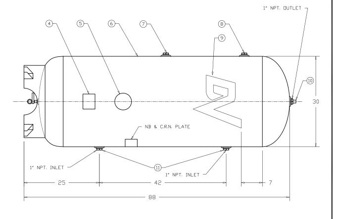
NOTE: 200 PSI. MAX. WURKING PRESSURE @ 650°F. NATIUNAL BUARD & C.R.N. APPRUVED. THREAD SEALANT MUST BE USED DN ALL FITTINGS. ALL FITTINGS MUST BE PLATED. TANK MUST BE PAINTED DV SYSTEMS GREY.
